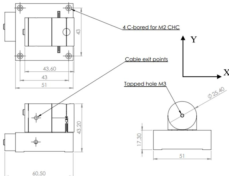
The axis of rotation are defined in the figure above. The bottom, rectangular, portion of the stage is the Y-axis and it gives a rotation about the Y-axis. The top, cylindrical, portion of the stage is the X-axis and it gives a rotation about the X-axis. The DB-9 connectors are labeled CHANNEL 1 (X) and CHANNEL 2 (Y) defining which axis of rotation that particular DB-9 corresponds to.
