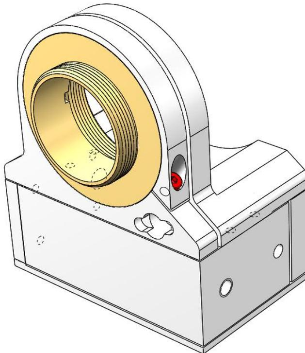
**Figure 1** : M2 blocking set screw (in red)
