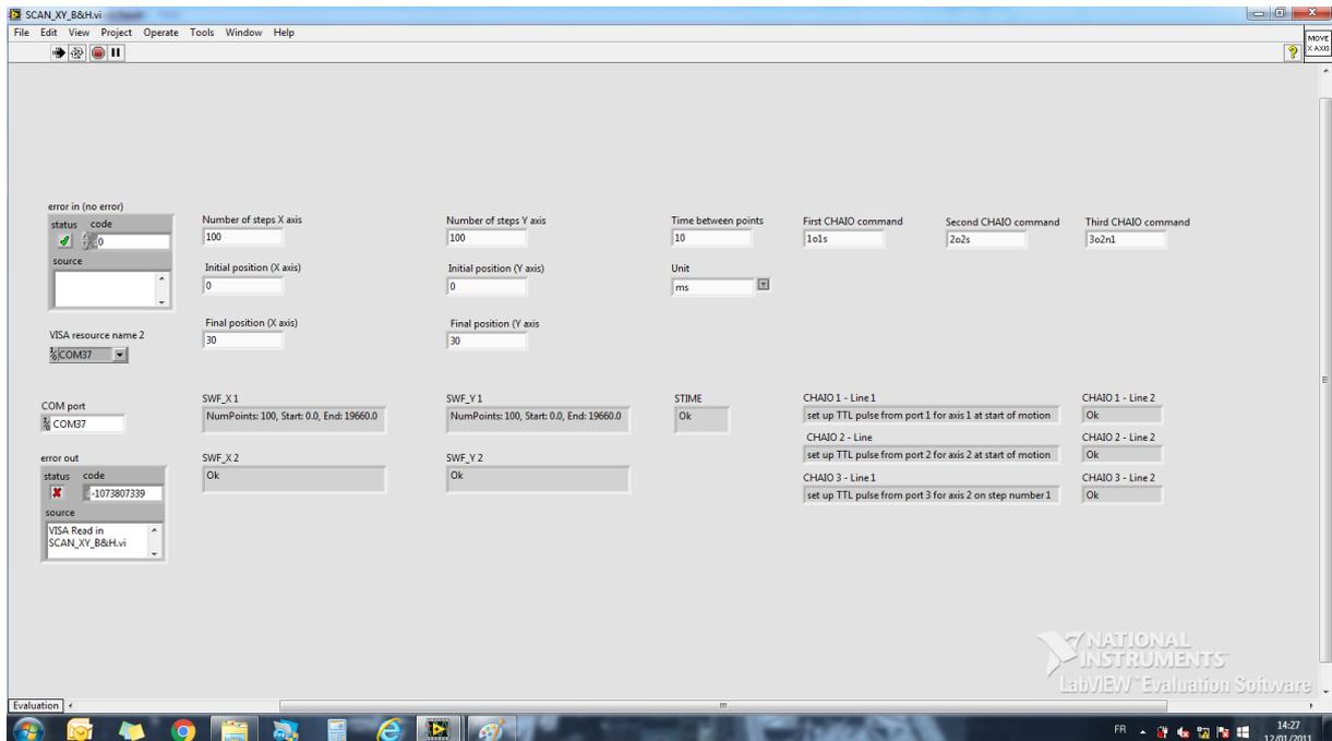
If you press the “RUN CONTINUOUSLY” button, the XY scan will be done again and again until you press the “STOP” button.
