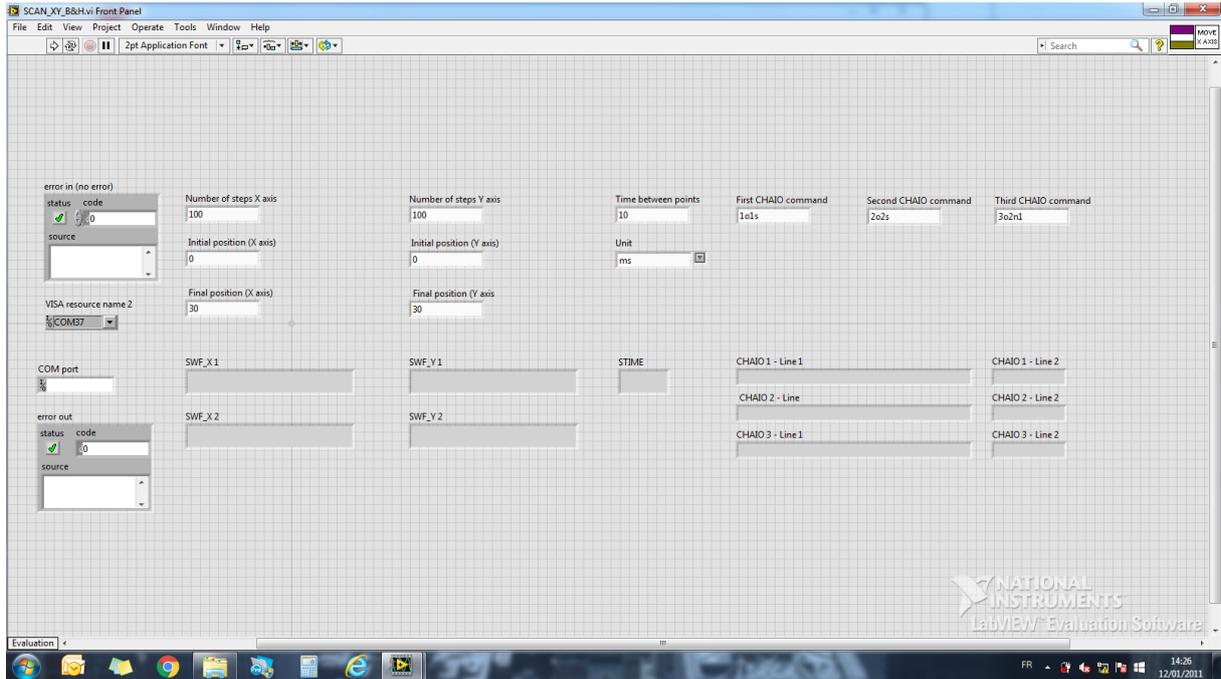
If you press the RUN button, all the commands will be sent, the buffer will be read. The scan will start and the TTL will be sent when they need to be. Please note that in that case, the XY scan will be done only once.
